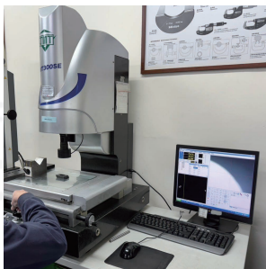
2.5D Vision Measuring System
