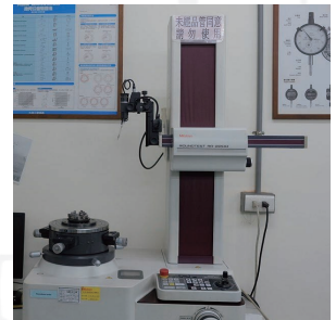
Roundness Measuring Instrument
