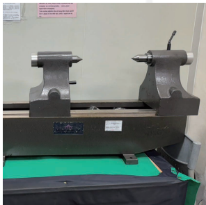
Double-Center Concentricity Gauge
