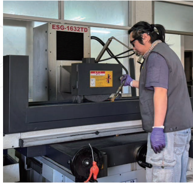
High-Precision Surface Grinder
